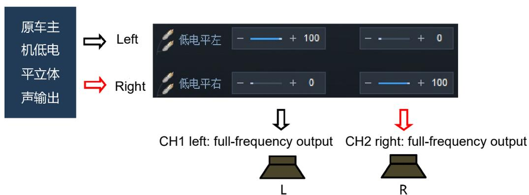
Example 2: active two-way frequency mixing input at high level from main device of original vehicle and stereo full-frequency output.
