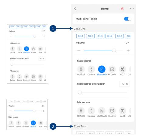
Click the "Multi-Zone Toggle" on the "Home" page interface to open the sound zone setting operation. The front and rear sound sources of Zone One and Zone Two can be matched. For instance, set zone one sound field from CH1-CH6 and select "Hi.Level" as the main source. In zone two, set the rear sound field from CH7-CH12 and select "Optical" as the main source. This means that CH1-CH6 will play high level audio and CH7-CH12 will play through optical input.
