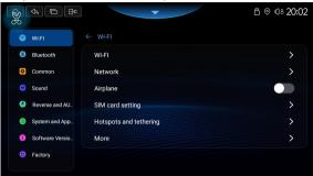
1. Tap [WIFI] key to enter the WIFI interface. Tap [ ● ] to turn WIFI on/off. After the WIFI is turned on, the searched signals will be displayed below; the [ 奈 ] behind each name indicates the strength of the WIFI signal. If there is a small lock beside the [ 奈 ] it indicates that the signal is encrypted. You need to enter the password before connection.
